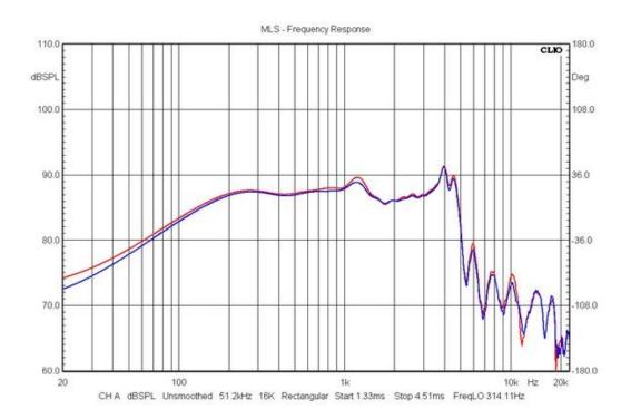
Frequency response from mounting the driver in a floorstander cabinet with front panel dimensions of  $190 \times 1000$  mm. Response from two drivers shown.
