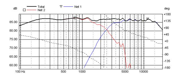
The smooth roll-off characteristic provides easy filtering at points of crossover around 2-3 kHz.
